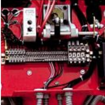
Example of the terminal board for the electrical connections for ENNE/EMME burner models
