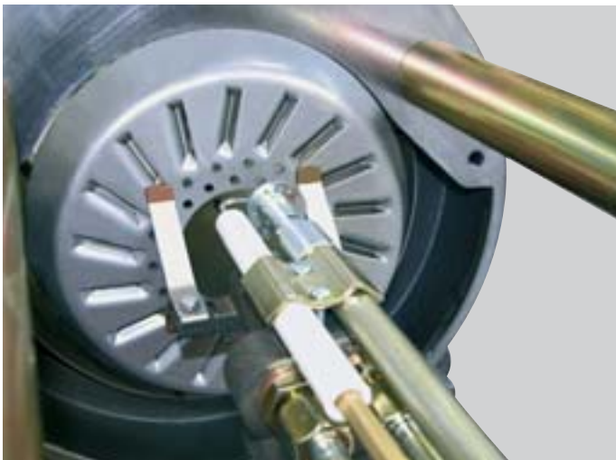
View of the electric-gas ignition system with LPG pilot burner
