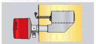
L2 - Angle configuration with combustion head developed in vertical in primary air duct
